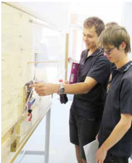
Year 11 physics students being taught how to calibrate the anemometer
